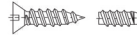
STAINLESS STEEL 304-A2 CSK PHILIPS (DIN 7982) TABLE - 7B CSK SLOTTED (DIN 7972) SELF TAPPING SCREW
