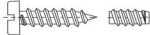
STAINLESS STEEL 304-A2 PAN PHILIPS (DIN 7981) TABLE - 7A PAN SLOTTED (DIN 7971) SELF TAPPING SCREW
