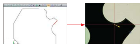
import CAD drawing, set the datum, establish coordinate system, then the software will automatically measure
