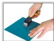
step 1: make grid cutting on surface
