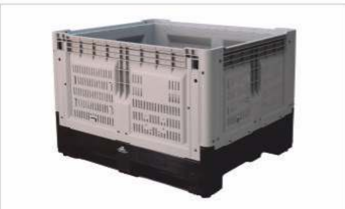
Model : CH1210800 | Outside Dimensions : 1200 (L) x 1000 (B) x 800 (H) All four side walls fold on base pallet, 2-way fork entry, 2-Bottom Runner Design.
