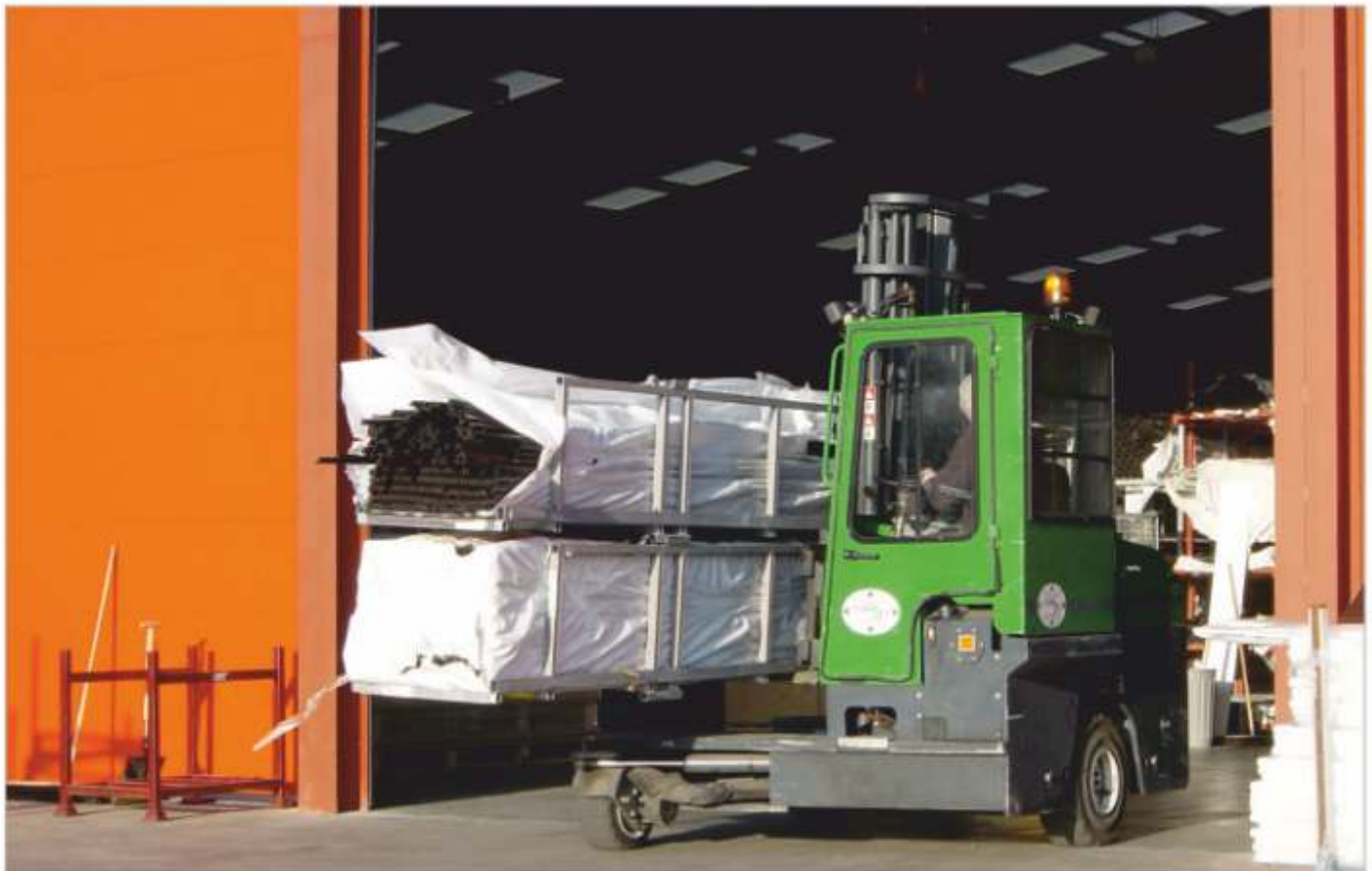
Moving long goods through doorways with sideways movement
