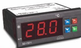
Dimension : 34.5x75mm Panel Cutout : 29x71mm
