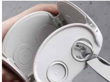
alternatively, a cable gland can be set after removing the elastic membrane and extension ring
