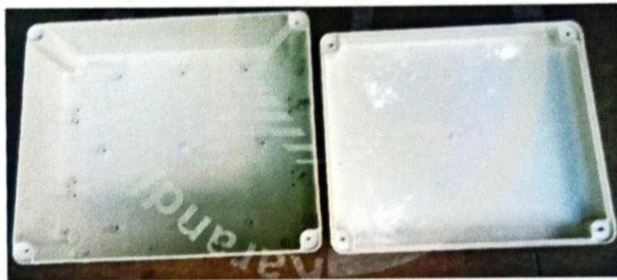
Picture2: No ingress of powder & water observed
