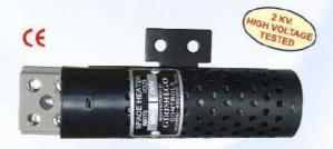
WORKING PRINCIPLE & FEATURES: The specially developed design incorporates a stainless steel sheathed cartridge heating element in perforated sheet metal enclosure. A black powder coated finish ensures rapid heat dissipation. A 2 x 2.5 mm porcelain terminal block is provided for electrical connection. Mounting Holes are provided at one side.
