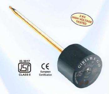
**PRINCIPLE OF OPERATION:** With temp rise, the principle of differential expansion of brass tube and a Nickel/Iron (inver) Rod is used to actuate a highly accurate snap action micro gap switch located in the head which makes it keep the temperature constant within the differential i.e. a single pole, single throw, normally closed circuit breaks (opens) on rise of temperature.
